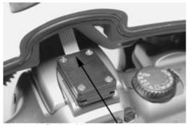
Picture C: flash cable connector
